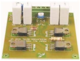
To change the current adjustment range select a new resistance for R6 and R7 using the calculation bellow. Remember that this will set the minimum current, you should select a minimum current below what is required so to allow for adjustment above and below the required current.
