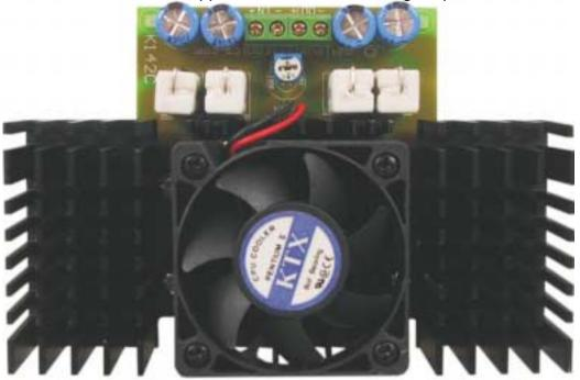
This kit is recommended for use with a 15-34V power supply and low voltage motors. The ideal situation would be a 33-34V supply with 2-4V motors. The K142C is adjustable to suit motors from around 0.5A to 2.5A. By changing the values of R6 and/or R7 lower and higher ranges can be achieved. See construction notes for details.
