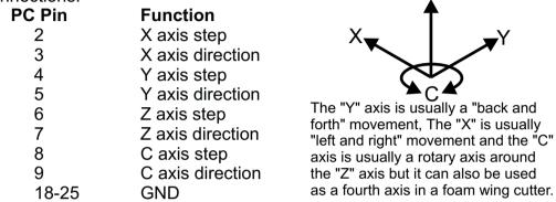
The other pins not shown here are often used for limit and home switches and will vary depending on the software you choose to use. In some cases they may not be needed at all or they can be disabled. The power supply in connection is required for the relays and 12VDC output. We recommend 9VAC or 12VDC from a power adaptor or other similar supply. The power supply 12VDC output is used to supply the logic (ICs etc.) of each of the K142B or K142D kits.
