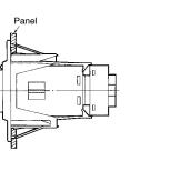
**Note:** Recommended mounting panel thickness: 1 to 3.2 mm.
