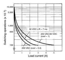
Note: A maximum current of 0.15 A can be switched at 125 VDC (cosf = 1) and a maximum current of 0.1 A can be switched if L/R is 7 ms. In either case, a service life of 100,000 operations can be expected. The minimum applicable load is 10 mA at 5 VDC (failure level: P).
