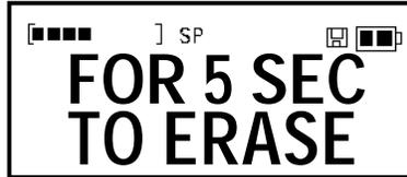
appear, the card needs to be formatted for use in the recorder. Press and hold Delete until you see the words ERASING CARD
