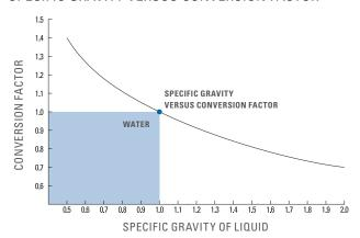
KEY: Conversion factor multiplied by the capacity of the nozzle when spraying water gives the capacity of the nozzle when spraying a liquid with a specific gravity corresponding to the conversion factor. This conversion factor accounts only for the effect of specific gravity on capacity and does not account for other factors affecting capacity.
