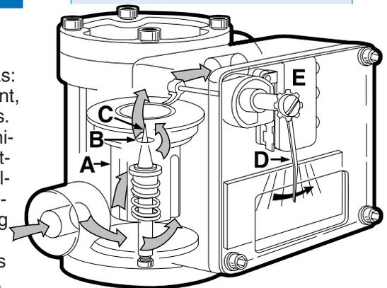
Fluid flow causes a spring-loaded piston **A** having a circular opening at its center **B** to move along the axis of a precision-tapered shaft **C**. This creates a variable orifice in direct proportion to the flow rate. The piston is mechanically linked to the readout pointer **D** and actuates switch **E** or a pot driven transmitter (not shown).
