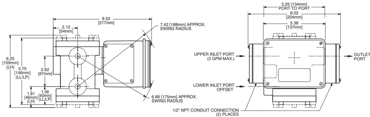
**Flanged Face to Face Dimensions for In-Line and Offset Installation**
