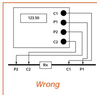
Most common cause of errors when making low resistance measurement are due to poor or inappropriate connection of the  $R_x$ . Connections should be clean, mechanically firm and free from oxides which can cause an insulating effect.
