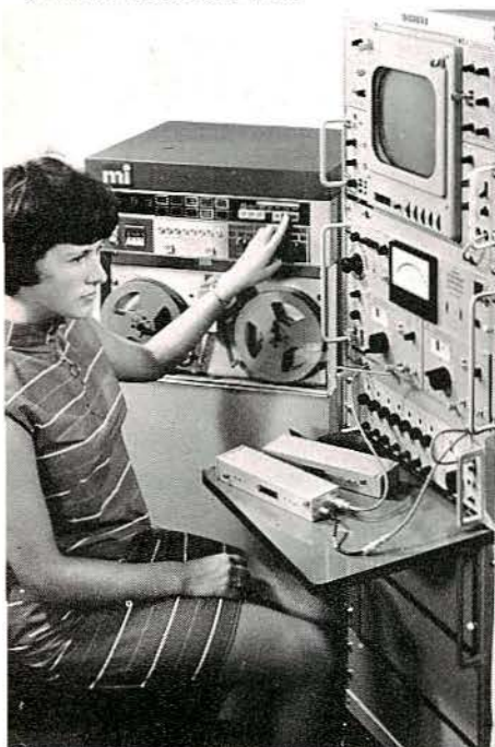
The "Autotest" response measuring system incorporating Siemens programmable instrumentation in use at the St. Albans factory of Marconi Instruments to check out filters from the large scale production of White Noise Test Sets.
