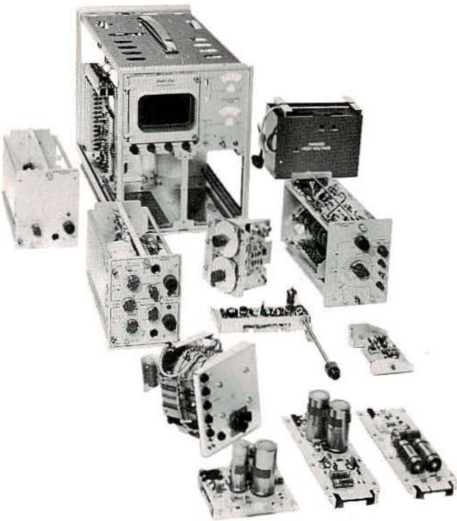
Electrical circuits take the form of easily detachable modules — see MODULAR CONSTRUCTION
