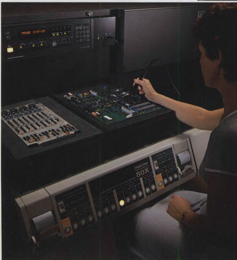
Automatic test systems 80X and 8080 speed the test and location of production faults on electronics.
