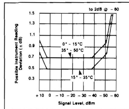
Figure 5 Model 1038-N10, NS20, and H/V Systems Waveguide Detector Accuracy from 26.5GHz to 40GHz
