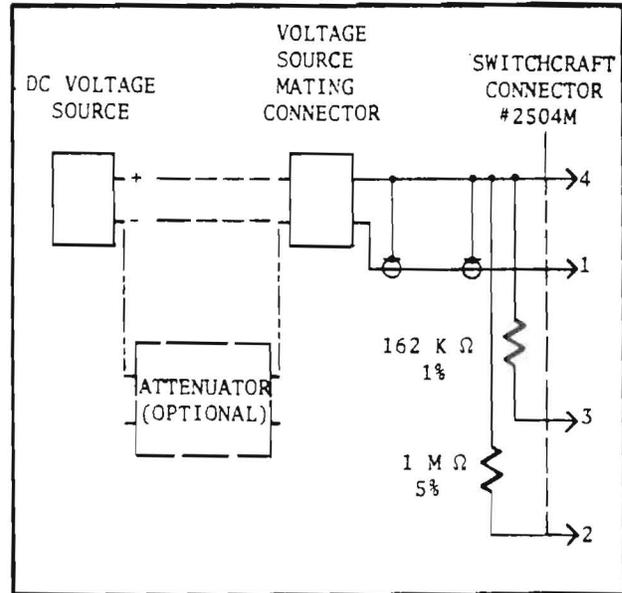
Figure 5-1. Modified Thermal Converter for Checking the Calibrator Output
