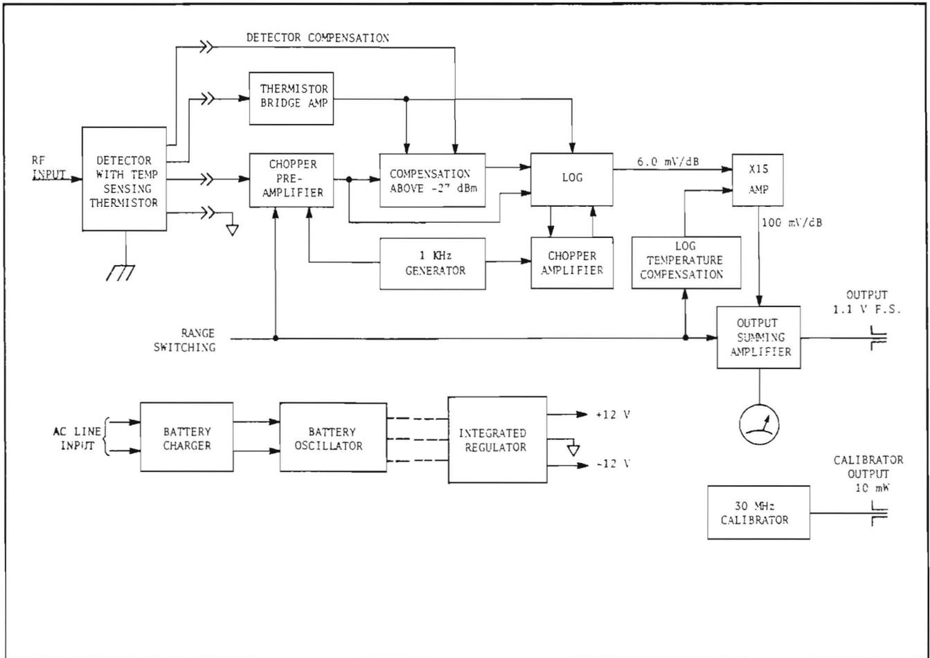
Figure 4-1. Model 1034A Block Diagram
