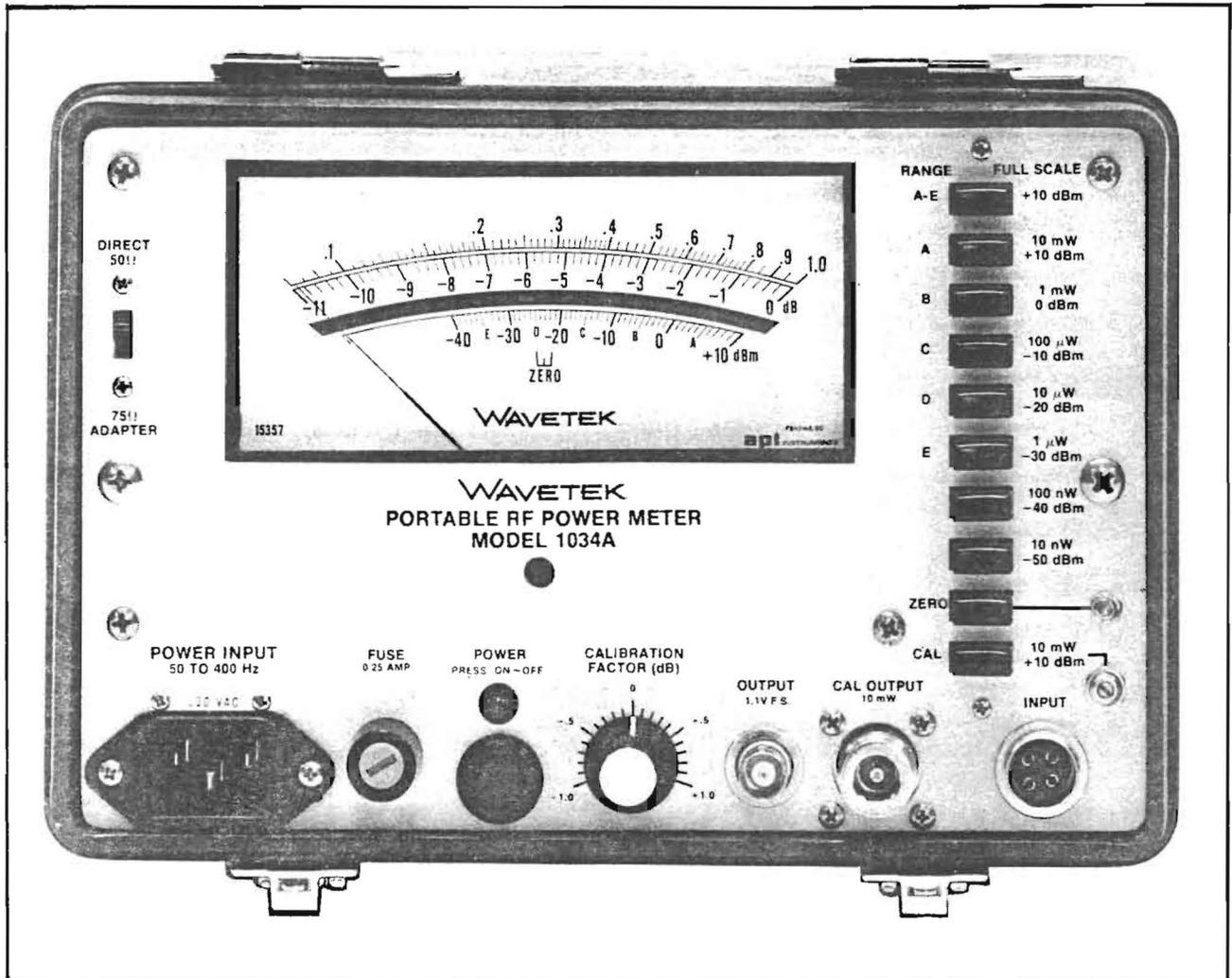
Figure 3-1. Model 1034A Front Panel
