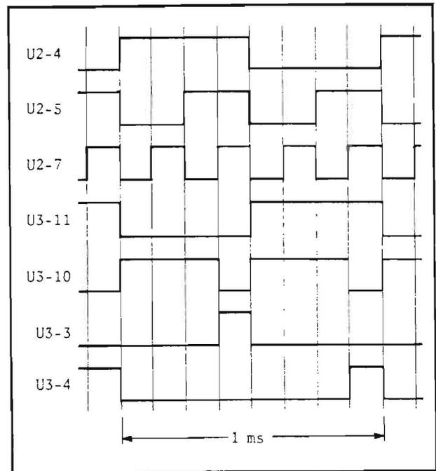
Figure 6-1. Chopper Circuit Timing Diagram
