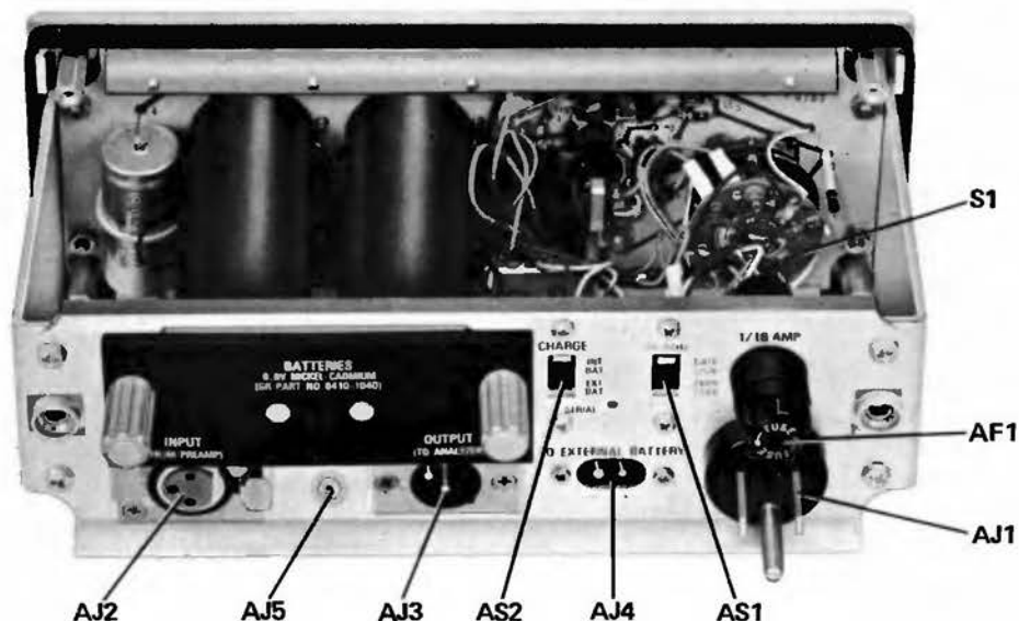
Figure 5-2. Controls and connectors on the rear panel of the Power Supply.
