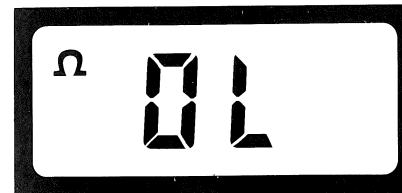
Figure 8. Display of Insta-Ohms Quick Continuity Indicator Symbol ( \Omega )
