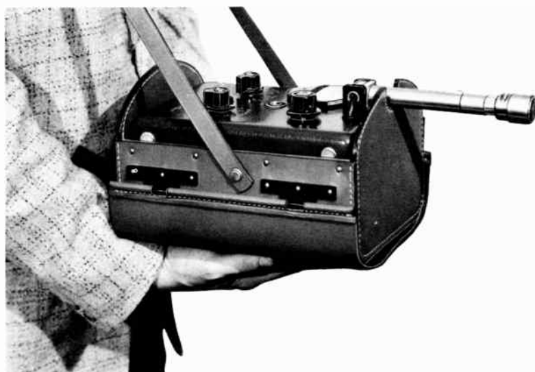
Figure 5-4. Hand-held operation of the sound-level meter.
