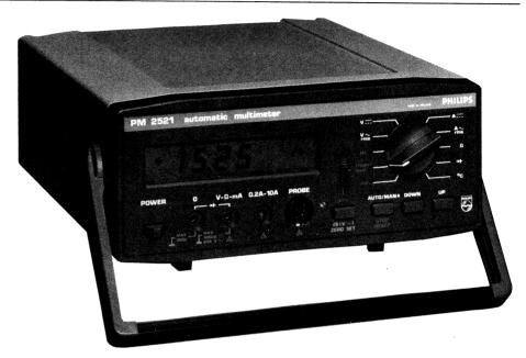
will then indicate the value, directly in dB, with 1mW into  $600\Omega$  as the 0dB reference. By applying the previously described relative reference technique, any desired "zero" point may now be selected and the measurements will be shown as a dB gain or loss. The fast auto-ranging allows for direct ratio measurements between 1mV and 600V.
