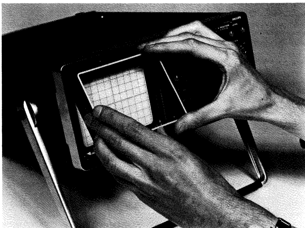
Fig. 3.5. Removing the screen bezel and the contrast plate
