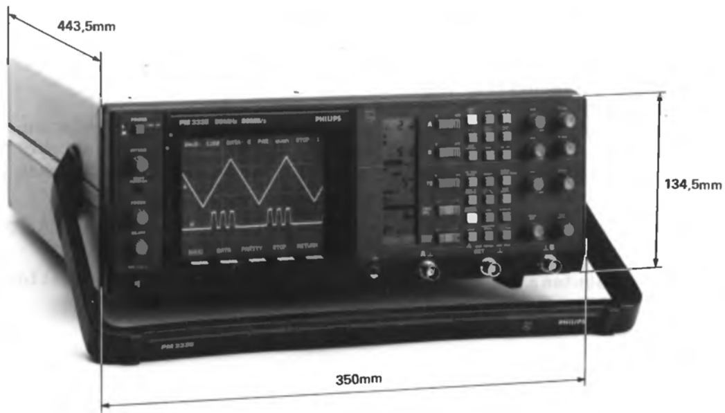
Figure 2.1 Dimensions of oscilloscope PM3335.
