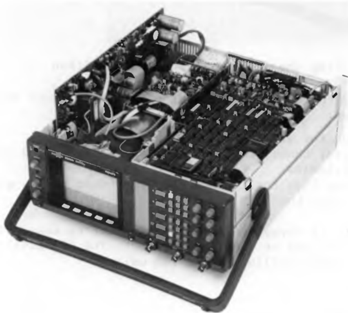
Figure 16.2 Power supply unit in service position.
