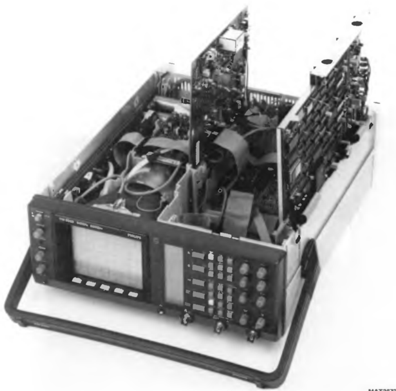
Figure 16.4 Measuring digital unit A9 and time base unit A4 in upright position for measuring in working condition.
