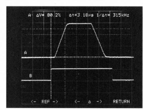
Phase measurements between channels are quickly and accurately made thanks to the extensive cursor facilities and the simultaneous acquisition on both channels. Without this simultaneous sampling the timing difference between the channels would result in measurement faults.
