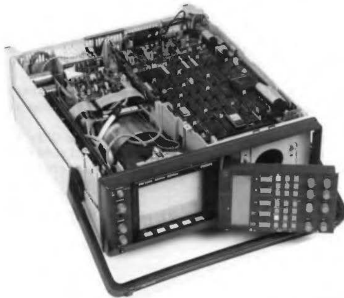
Figure 16.3 Measuring the front unit working condition
