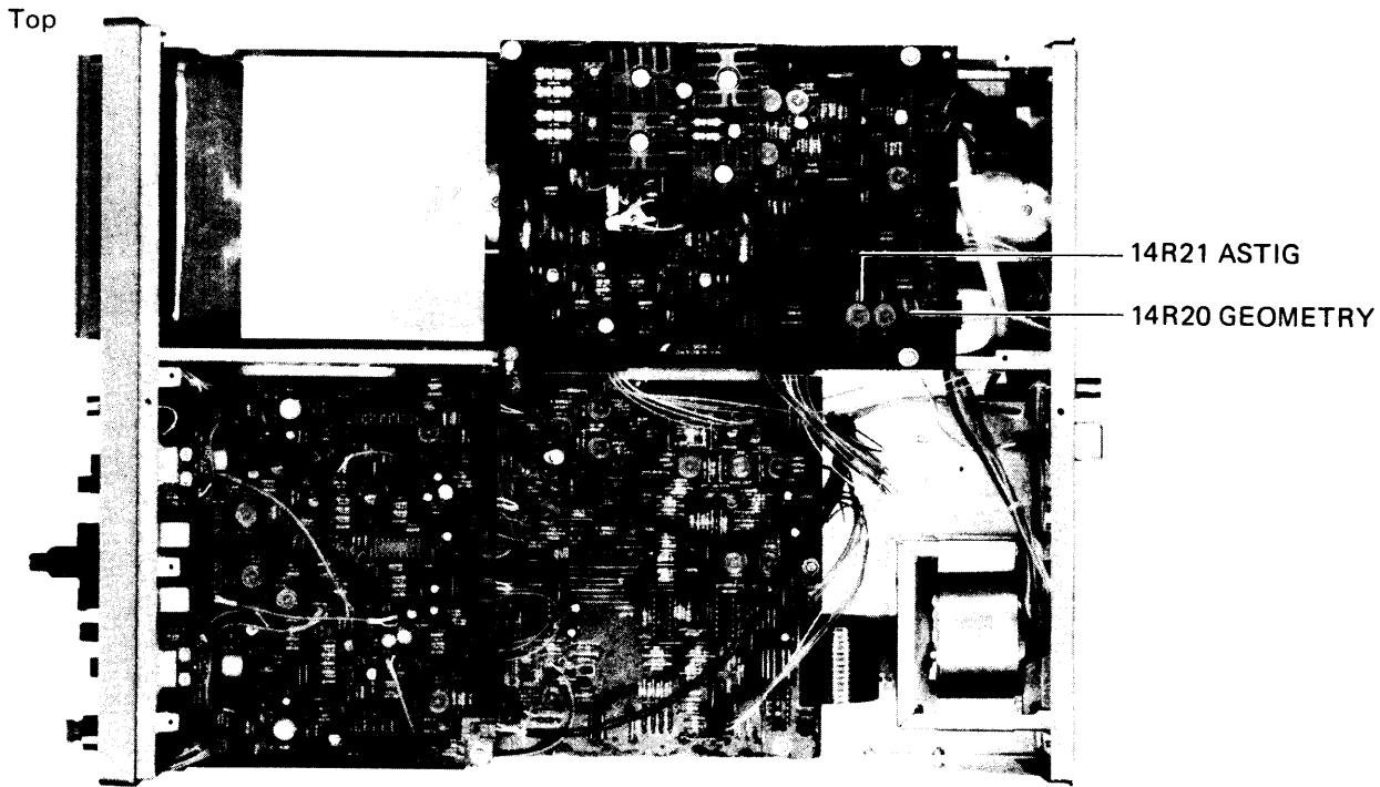
Figure 6-7-2. Adjustment and Testpoint Locations (POWER SUPPLY and CRT)
