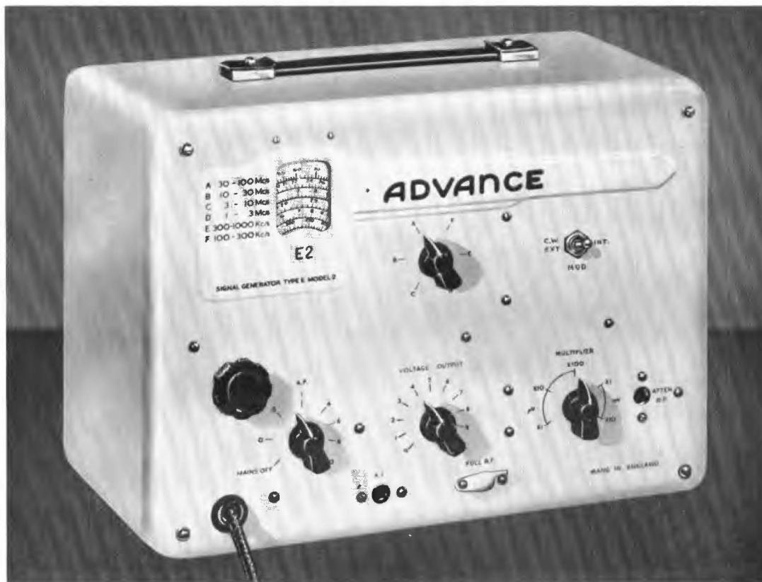
**T**HE most widely used instrument in its sphere, the type E2, which operates entirely on *fundamental* frequencies, is characterised by its exceptionally low R.F. leakage, which even at 100 Mc/s, is less than three microvolts. In addition to internal modulation at 400 c/s, 30%, it may be modulated from an external source to give 0.80% modulation up to 4 kc/s, and 0.40% modulation up to 10 kc/s. The input impedance is 50 k ohms so that little power is required for modulation.
