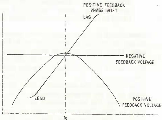
Fig. 2 Conditions for Oscillation
