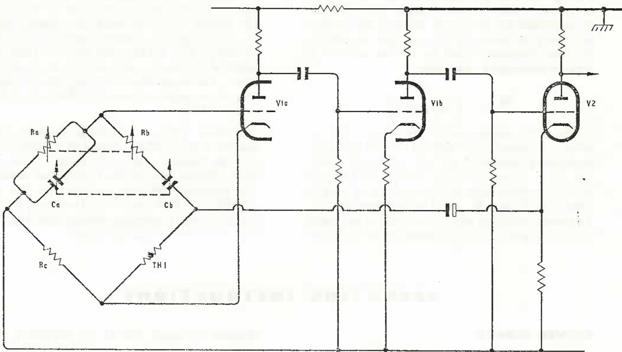
Fig. 1 Basic Wien Bridge Oscillator
