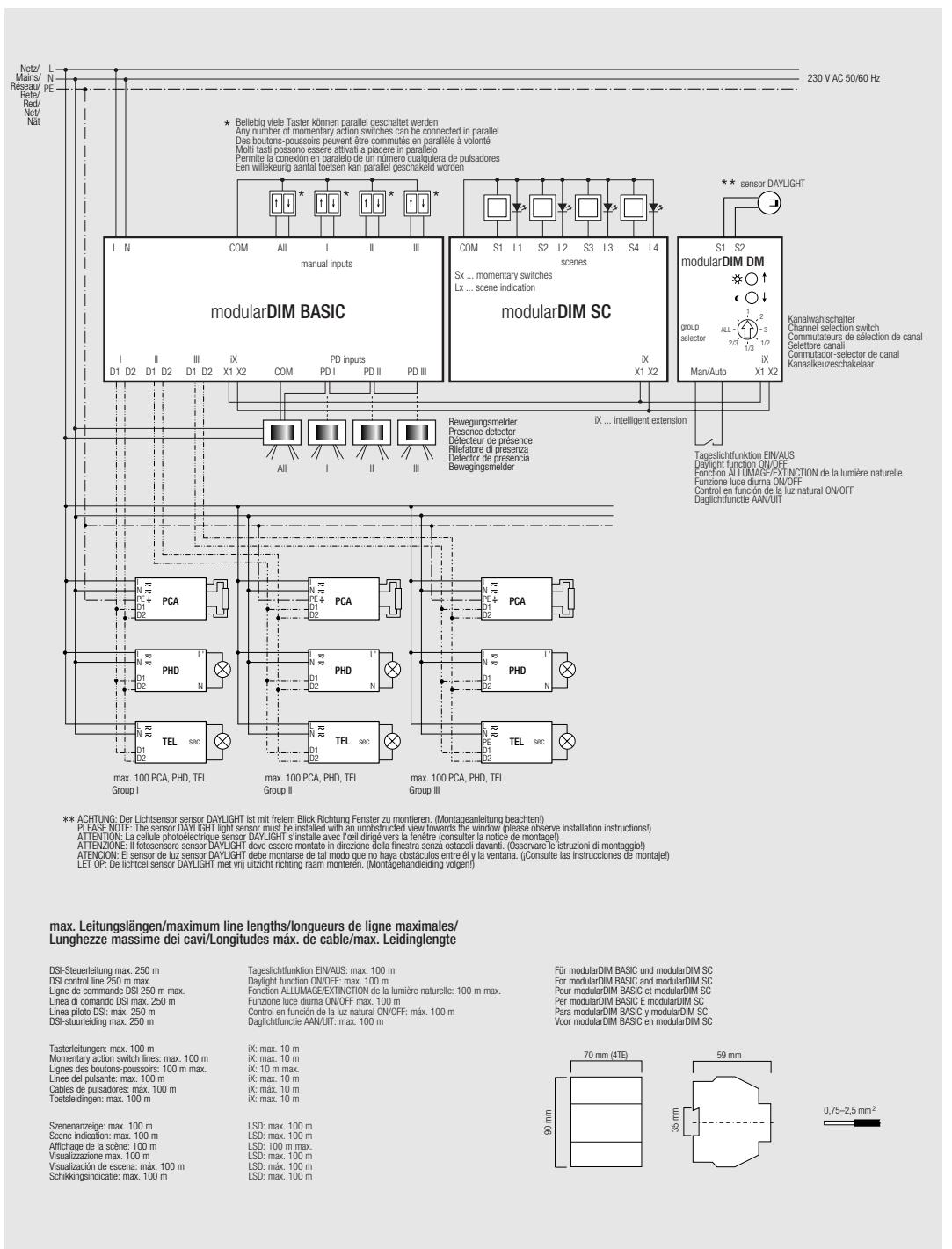
**UK** The modularDIM light control system consists of the core module, the modularDIM BASIC, which works as the group controller, and the extension components modularDIM SC for saving and calling up of lighting scenes and the daylight control device. The daylight-dependent control (modularDIM DM) of up to 3 light groups (continuous row systems) occurs depending on the daylight available in the room that is detected by means of the light sensor "sensor DAYLIGHT".
