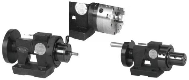
The GSG Zero spindle offers various methods of holding a part on the outside feature during rotation. The charts show the 4 major methods: Collet, 3-4 Jaw Chuck, and external off Lead Lock. These methods can be combined with various measurement methods and provide the user with a robust and repeatable way of inspecting ovality, run-out, diameter and true position of round parts.
