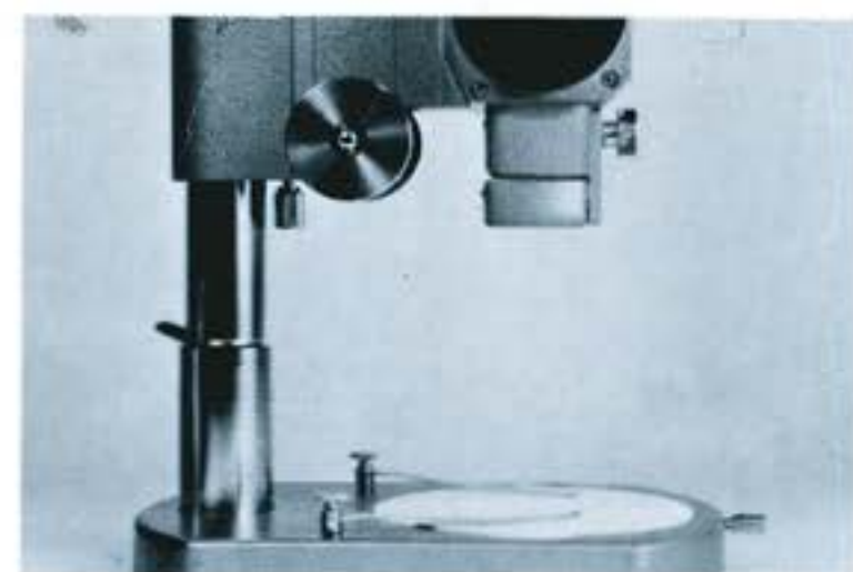
3. Large working distance - up to 86 mm with 1X objective, 45 mm with 2X objective.
