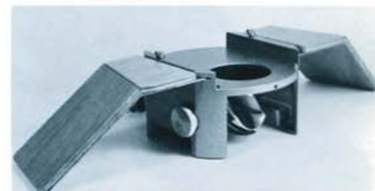
10. Trans-illuminator base provided with 20 watt bulb.
