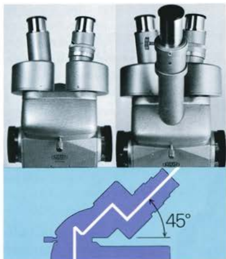
1. Binocular tube for X with 45° inclination. Detachable and reversible 180°. Trinocular tube for X-Tr.
