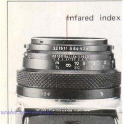
In infrared photography, some adjustment must be made in the focus in order to retain sharpness on the film because the invisible infrared Pays are longer in wave length than the visible rays used for focusing. For infrared photography--
