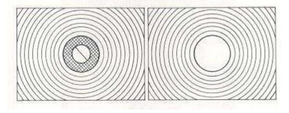
A focusing screen with matte center plus full-area fresnel lens outside the center spot is also available.
