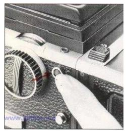
If the green-colored battery check lamp lights up when the battery check button is depressed, the battery is loaded properly and there is sufficient power for electronically-con trolled operations.
