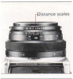
A. Distance scales on the Bronica lenses for the ETR can be used for setting the focus on the required distance or finding the distance actually focused. Simply rotate the focusing ring and set the required distance opposite the green colored index, which will adjust the lens for the required distance.
