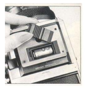
B. Depress the battery chamber button with your finger while, at the same time, moving the battery chamber cover in the arrow-indicated direction and the cover will come off.
