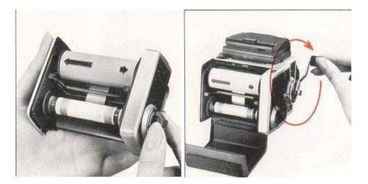
E. When the fresh film spool is properly loaded in the top spool holder, draw out the leading end of the film and turn it across the film pressure plate (on the front side of the insert). After running it down to the lower end, turn it over to the empty take-up spool. Insert the leading end of the film into the slit of the take-up spool and wind slightly so that it is securely engaged.
