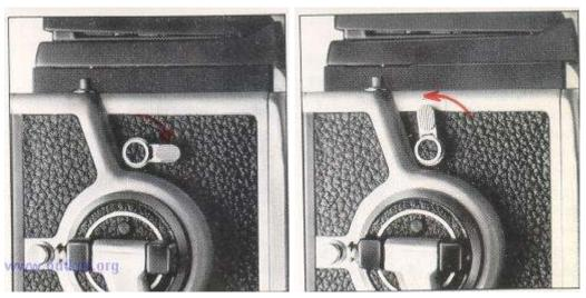
A. To make multiple exposures rotate the film winding crank (to advance the film and cock the shutter) and then turn the multiple exposure lever in the clockwise or arrow-indicated direction. When set in this manner, the shutter can be released and cocked any number of times, without advancing the film.
