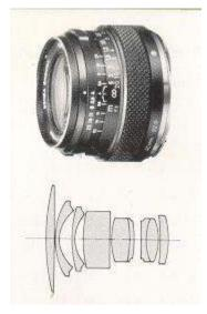
Zenzanon E 40mm F4 Lens construction: 9 elements 7 groups Angle of view: 82°30' F/numbers: 4 to 22 Diaphragm: Fully automatic Minimum focus: 40cm (1.3 ft.) Electronic leaf shutter: Seiko #O Shutter speeds: 8 sec. to 1/500 sec. plus T (time exposure) Filter size: 62mm screw-in type Length: 62mm Weight: 478 grams (1.04 lbs.) Equivalent 35mm focal length: 25mm
