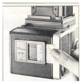
Upon loading the film, tear off the end flap from the empty film package and insert it in the film type indicator frame. This will help you keep track of the film loaded in the film back and should prove useful when two or more film backs are used, with different types of films.
