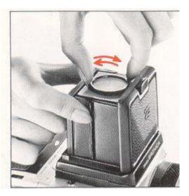
**C.** The standard magnifier supplied with the waist-level finder has a power of--1.50 diopters, which can be exchanged for others with Powers of +1.50, +0.50, -0.50, -2.50, -3.50 and -4.50 diopters. These optional accessories should be purchased to suit the user's eyesight, if necessary. Simply rotate the magnifier frame in the counter-clockwise direction to unscrew.
