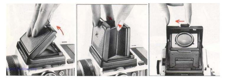
**A.** The focusing hood of the waist-level finder is opened by pushing or pulling up on the focusing hood/magnifier catch at the rear end of the folded waist-level finder.
