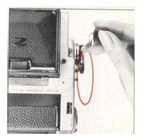
H. Close the back cover, by pressing it strongly against the base of the film back, as illustrated. The back cover will automatically lock and close.
