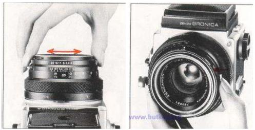
A. The aperture ring is rotated, in either direction, to set the required f/number opposite the white index dot. The aperture ring click-stops at the numbered settings. Intermediate settings are also possible.
