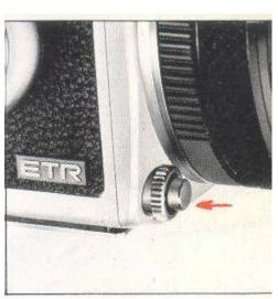
**B.** Safety Lock The shutter release button can be locked to prevent accidental operations, by simply rotating the locking ring 55° in the clockwise direction. This will place a red dot on the side, indicating that it is locked. To release the safety lock rotate the locking ring in the counter-clockwise direction which will place the dot diagonally lower. The shutter cannot be released, in the following cases:
