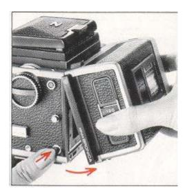
The camera body and film back are fully coupled at all times, upon connection. When film backs are interchanged, the shutter cannot be released if the shutter is not cocked or the film is not advanced or both. Upon changing the film back, therefore, always turn the film winding crank completely one time. If the shutter is not cocked or the film is not advanced, the incomplete actions will take place when the film winding crank is rotated.
