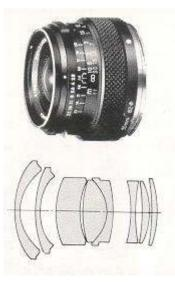
Zenzanon E 50mm F2.8 Lens construction: 8 elements 7 groups Angle of view: 70° F/numbers: 2.8 to 22 Diaphragm: Fully automatic Minimum focus: 50cm (1.6 ft.) Electronic leaf shutter: Seiko #0 Shutter speeds: 8 sec. to 1/500 sec. plus T (time exposure Filter size: 62mm screw-in type. Length: 62.5mm Weight: 464grams(1.01 lbs.) Equivalent 35mm focal length: 30mm
