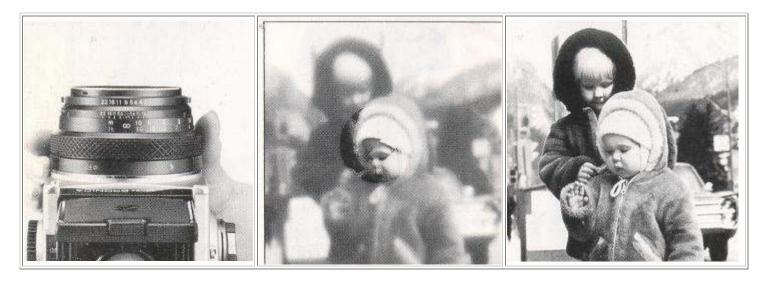
A. The lens is focused on the subject, by rotating the focusing ring in either direction, while checking the effect on the microprism / split-image rangefinder spot in the center of the focusing screen (standard type).
