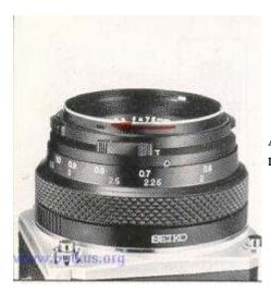
A. Time exposures are made with the time exposure lever on the lens, regardless of the setting on the shutter speed scale.
