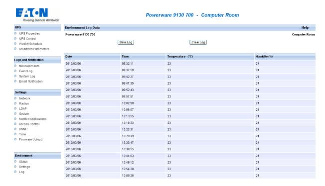
The two environment sensor measurements: Temperature and Humidity are recorded at an interval defined by the Environment log interval in the <u>System settings</u> page.
