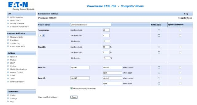
The environment sensor measures temperature, humidity and gives the status of the 2 contacts (used for door, alarms or generator unit).
