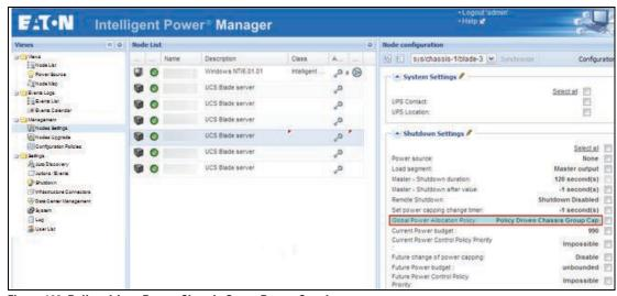
Figure 193. Policy-driven Power Chassis Group Power Capping
