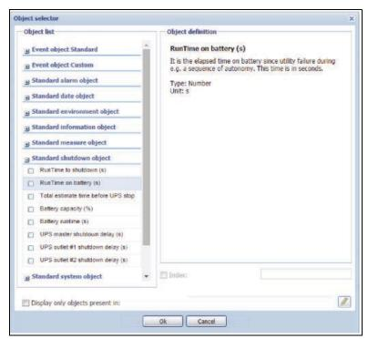
Figure 222. Object Runtime on Battery
