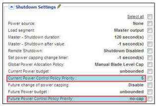
Figure 195. Shutdown Settings-Current Power Default Setting (Priority 5)
