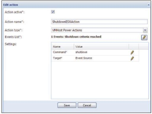
Figure 220. Create Shutdown ESXiAction
