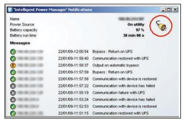
Figure 47. Alarm Notification Box with System Tray Icon
