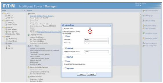
Figure 12. Remove Duplicated Nodes Automatically
