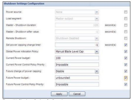
Figure 191. Shutdown Settings Configuration
