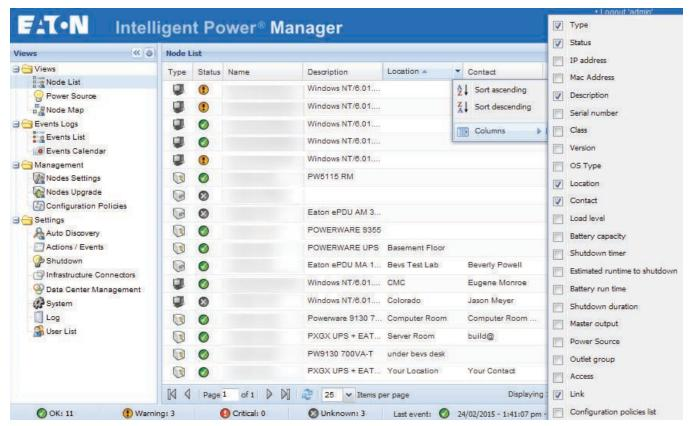
Figure 49. Adding Columns in Node List View
