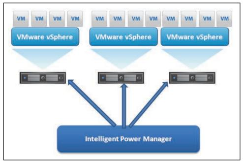
Figure 90. Eaton IPM Connected to ESX/ESXi to Protect VMware Infrastructure (Without vCenter)
