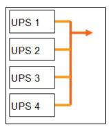
Figure 150. Parallel Redundancy Schema
