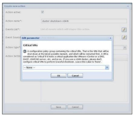
Figure 42. Create Action for vSAN Cluster Shutdown
