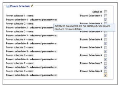
Figure 83. Advanced Parameters Not Displayed
