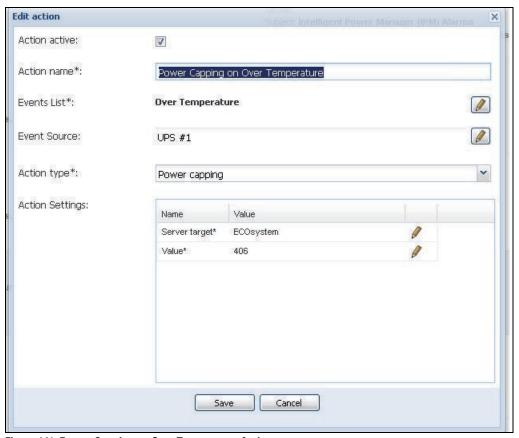
Figure 141. Power Capping on Over Temperature Action
