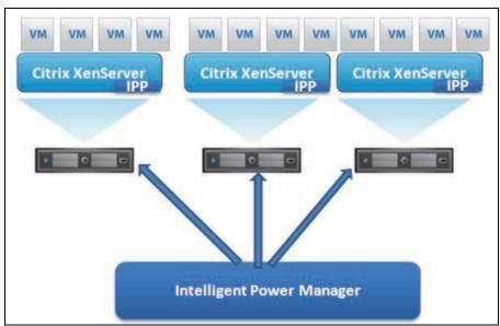
Figure 107. Eaton IPM Connected to XenServers (Triggers XenMotion and Eaton IPP Running on XenServer Infrastructure)
