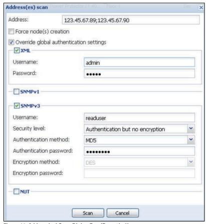
Figure 11. Address(es) Scan Dialog Box (Example 2)
