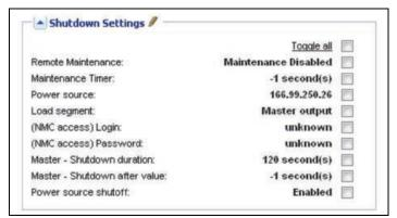
Figure 145. Shutdown Settings for VM Host with Eaton IPM
