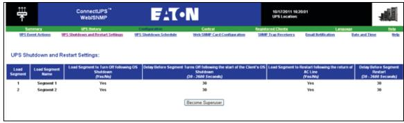
Figure 158. UPS Shutdown and Restart Settings
