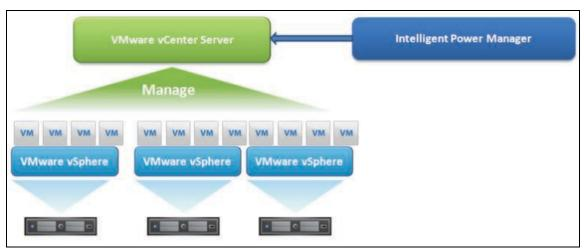
Figure 89. Eaton IPM Connected to vCenter to Protect VMware Infrastructure
