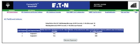
Figure 161. UPS Shutdown and Restart Settings
