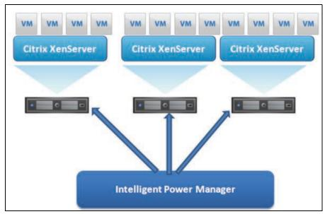
Figure 108. Eaton IPM Connected To XenServer to protect the XenServers
