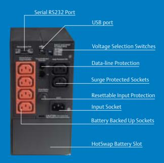
**Battery Backed Up** sockets offer surge protection in addition to battery autonomy in case of a power failure. Surge Protected Only sockets offer surge protection for devices that do not need battery back up in case of power failure (InkJet Printers, Scanners, Multimedia Equipment).
