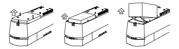
Changing the batteries in your UPS is a safe and easy procedure. Since the battery is isolated from the AC input you may leave your UPS and computer or other equipment on during the following procedure. Please note that if you choose to leave the UPS on when the battery is removed, it will not be able to power your equipment if a power failure occurs. Please read the cautions in section 6.1 before performing the following steps.
