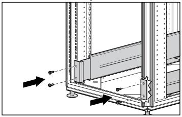
6. Install the rear stabilization bracket.
