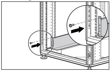
5. Insert the screws into the back of each rail and through the cage nuts that were installed in step 3.
