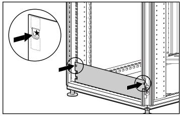
3. Use the cage nut tool to install the cage nuts in the rear rack-mounting rails.
