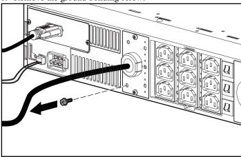
Attach the grounding cable and secure the ground bonding screw.
