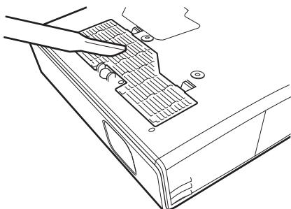
When it becomes difficult to remove the dust from the filter with a vacuum cleaner, remove the air filter and wash it.
