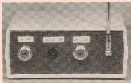
This rear view of the unit shows the RF and DC connectors, and also the base of the rod antenna.
