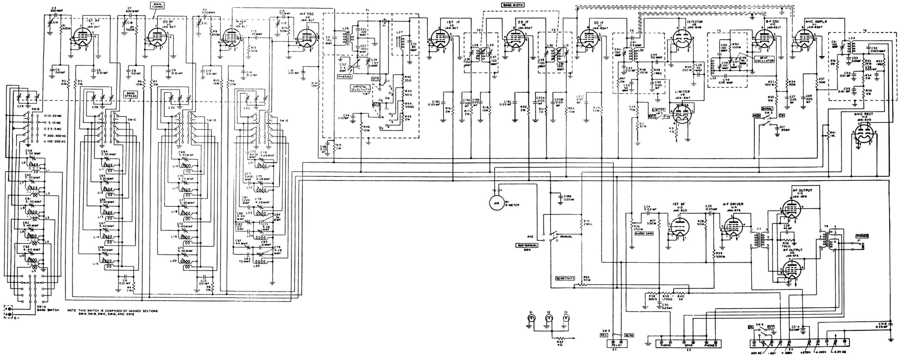
Schematic Diagram, Receiver BC-779-A, B
