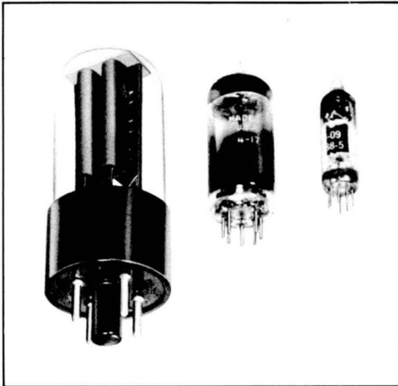
*Subminiature Tube Compared with Standard Tube*
