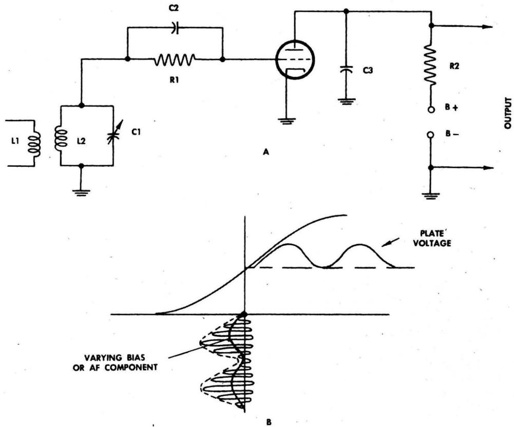
Grid Leak Detector and Response Curves
