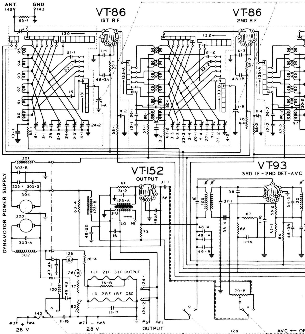
Schematic Diagram, Receiver BC-348 AL
