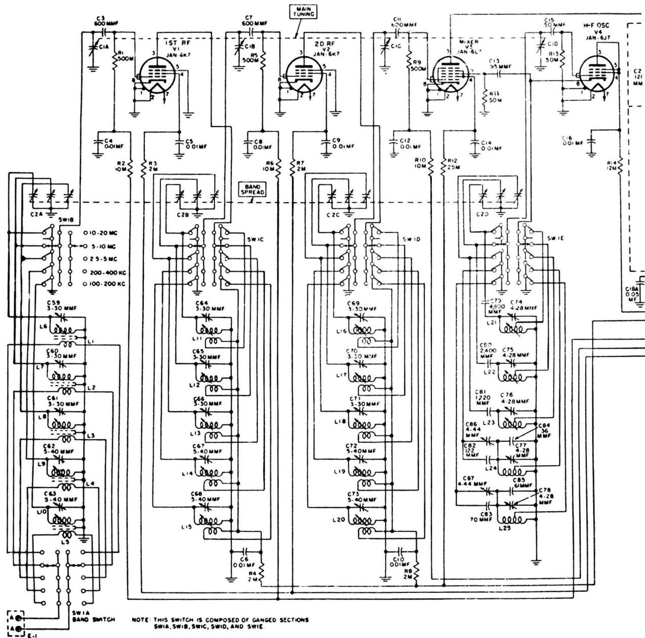
Schematic Diagram, Receiver BC-779-A, B
