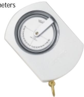
8025-75 0  $\pm$  90° scale on the left, 0  $\pm$  150% scale on right; reads directly to 1/6 of one degree or 1/5 of one percent; skylon case.
