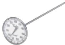
As accurate as mercury thermometers, but without the need for safety precautions to avoid potential toxicity; measures temperature via a bi-metallic coil attached to an indicator needle.
