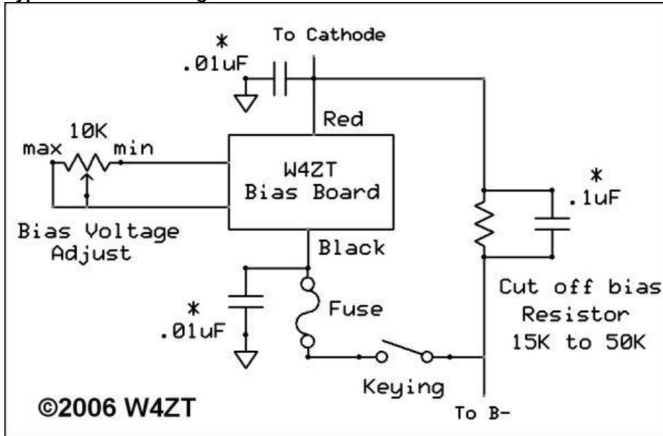
The 10K potentiometer, R1, provides a bias adjustment range of approximately 3.5 to 39 volts. For initial installation the potentiometer should be set for maximum bias to insure you start your adjustment at the lowest plate current. Fuse the circuit just above the maximum expected plate current.
