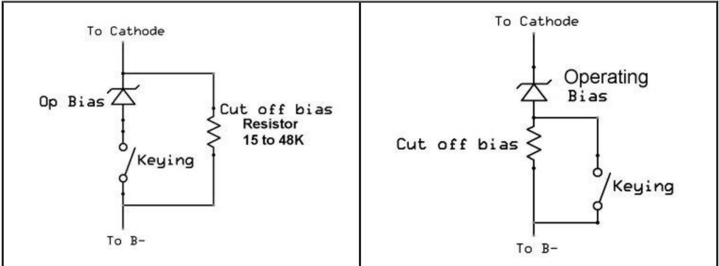
Typical connection diagram for the bias board
