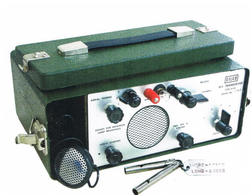
Figure 1 Type 6801 SSB set, 5 channels, 100 watts PEP
