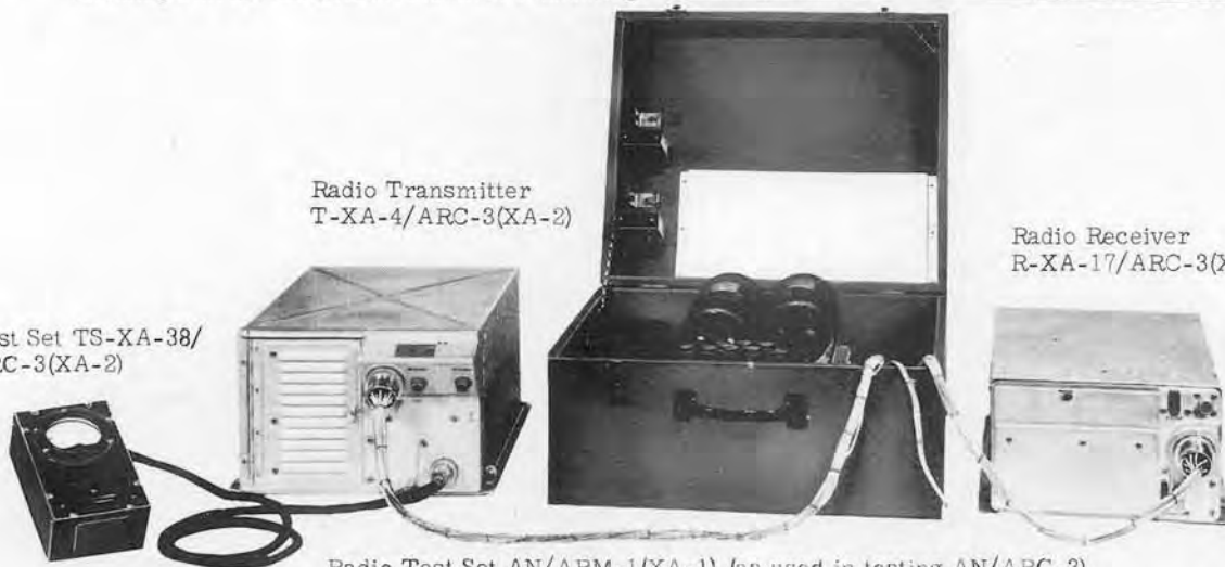
Radio Test Set AN/ARM-1 (XA-1) (as used in testing AN/ARC-3)
