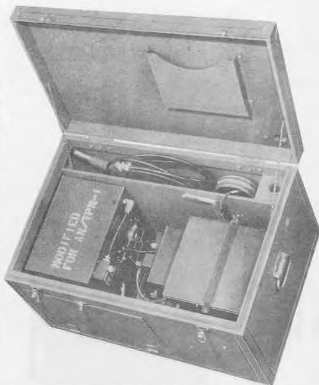
AN/TPN-1 packed in Case CY-21/TPN-1 is air transportable and easily assembled.
