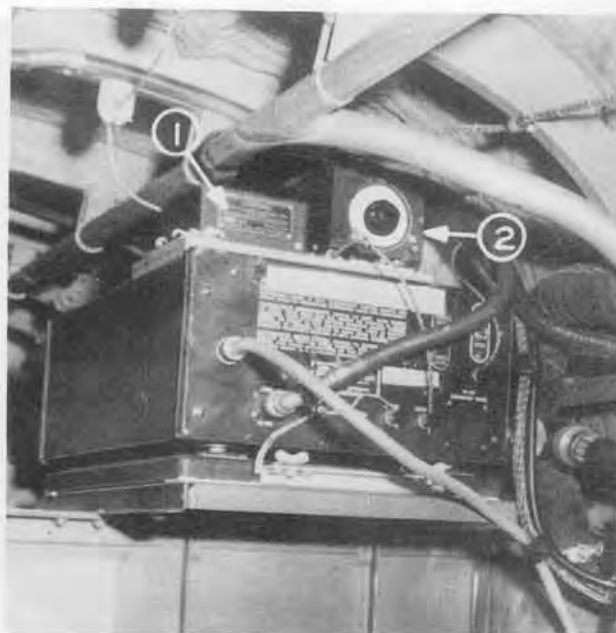
Installation photograph indicates (1) Relay RE-1/ARR-1, and (2) Radio Receiver R-1/ARR-1
