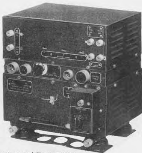
Radio Receiver and Transmitter *RT-1A/APN-2 on Mounting FT-416-A
