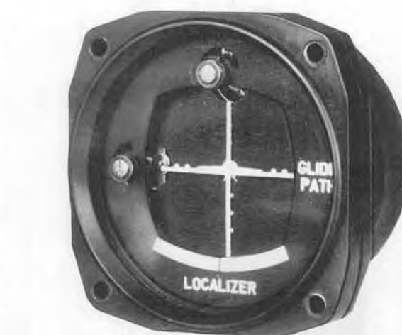
The Vertical Pointer of Indicator I-101 records position of aircraft with regard to alignment to runway.
