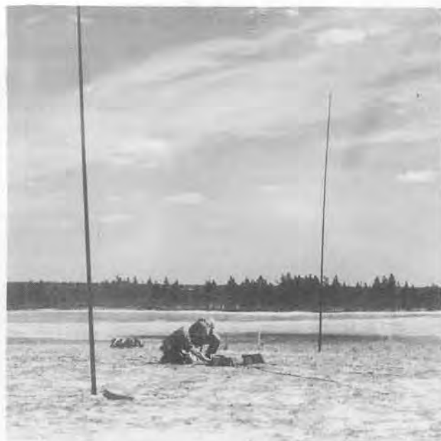
Radio Set AN/CRN-4 dropped with pathfinder troops may be set up in 30 minutes.
