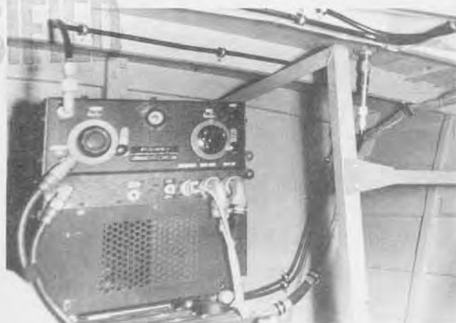
Receiver-Transmitter RT-21/APN-7 installed for operation.
