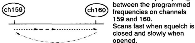
Channel scan and channel resume scan increases channels within a 5 channel range such as ch 1 to ch 5, ch 156 to ch 160, etc. in user channels; or all channels in the group of ITU channels
