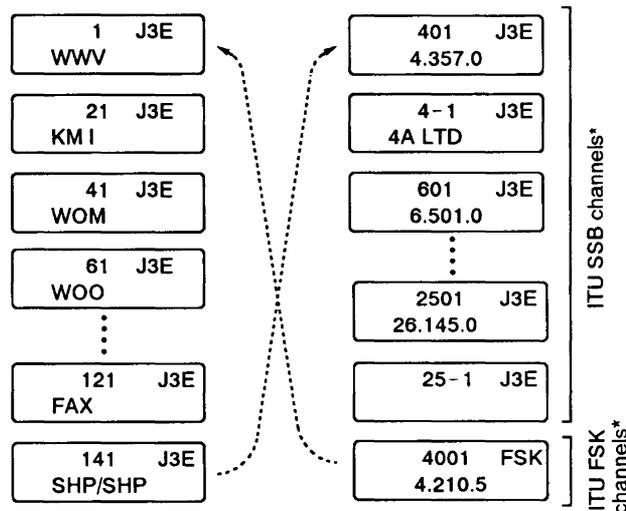
\*All ITU channels are not available with some versions and ITU FSK channels can be hidden using set mode. (p. 12)
