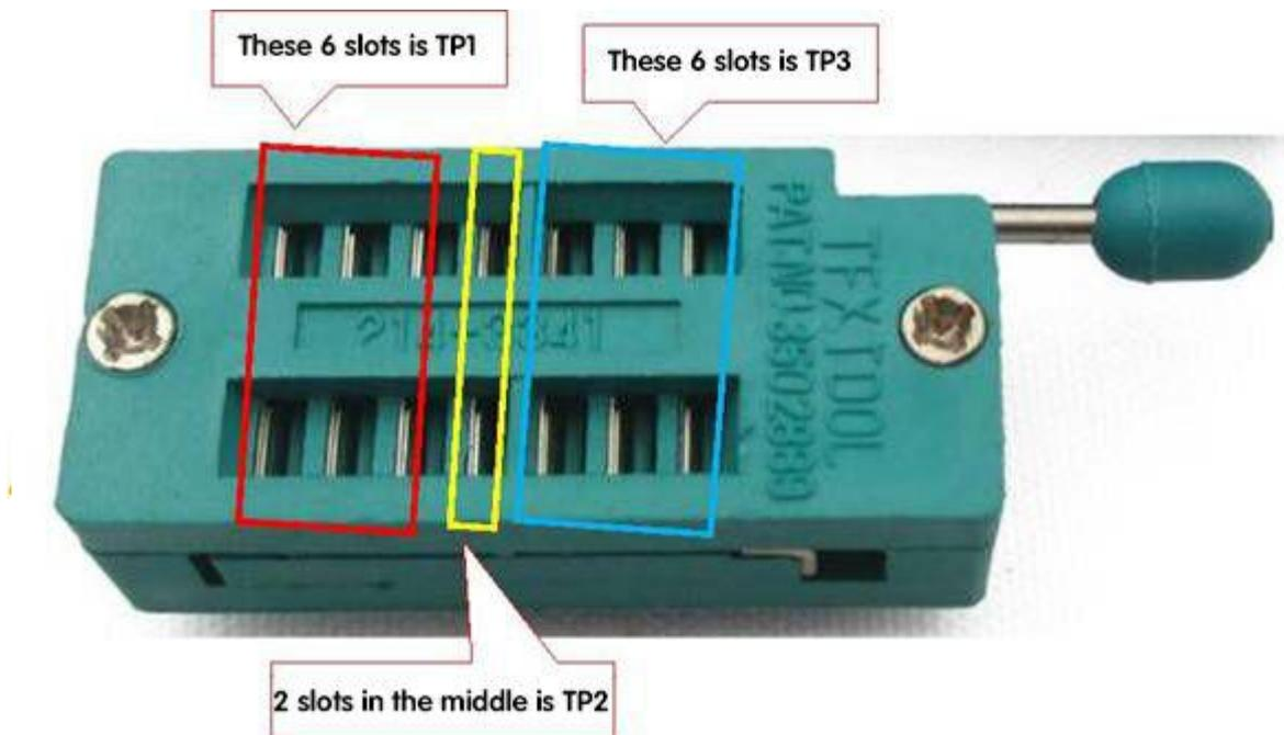
The test position of the patch element is on the right side of the test seat. There are above digital 1,2,3 , each representative TP1,TP2,TP3. Test only 2 pin components, pin no test order, 2 pins arbitrarily selected 2 test points. 3 pin device pins are placed in the three test points, pin no test order. After testing, pin name of the element and the location of the test point be identified automatically and displayed on the screen.
