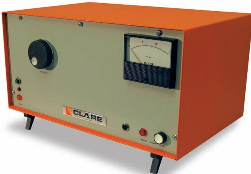
The A203 range of hipot testers is robust and simple to use. Each instrument is ideally suited to manufacturing or laboratory environments and offers high accuracy control, allowing continuous selection of voltage from 0 to 15kV AC from a 500VA transformer source. Output voltage is clearly displayed on moving analogue meters. Also available is a selection of features which includes current monitoring from a variable trip settings for over-current and audio-visual indication.
