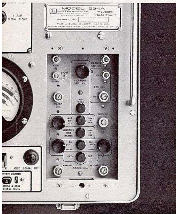
Controls for calibration and special tests are located in an auxiliary compartment. A hinged cover (not shown) covers the compartment during normal operation.
