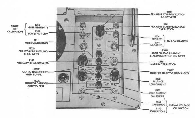
Figure 3 - Auxiliary Compartment
