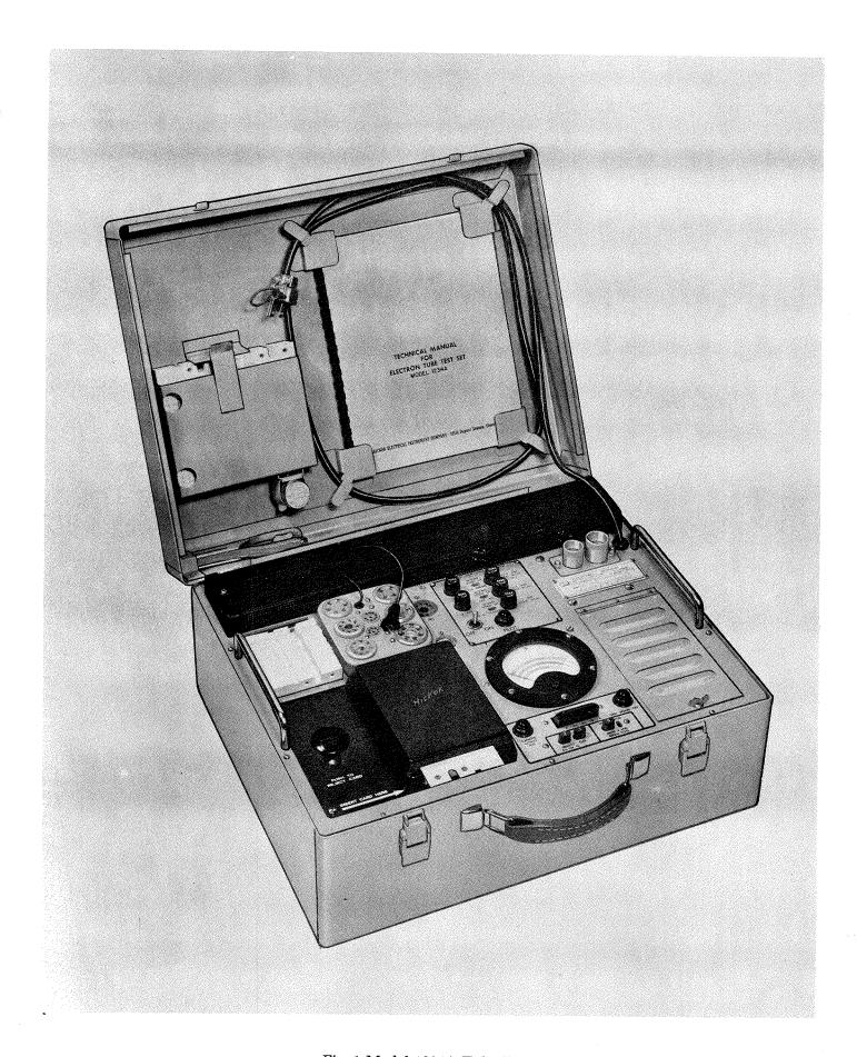
Fig. 1 Model 1234A Tube Tester
