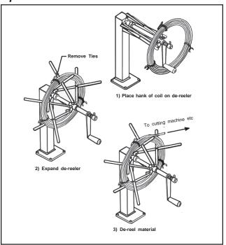
The CW10 shown used to de-reel. To reel material into coils or hanks reverse the operation shown.
