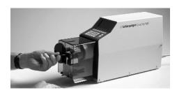
Sensor Activated Start Cycle: Some machines require a button or a footpedal to be depressed to activate the machine cycle. Others use a sensor that detects the cable end to begin the machine cycle. The "sensor type" is preferred by most operators because it requires one less operation compared to pressing a button or a footpedal. If it is a sensor type, verify that even your smallest cable can trigger it without the cable buckling.
