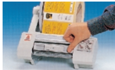
Push satellite roller down ...
