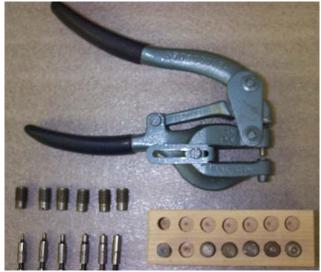
Lower anvils are classified into groups (A,B,C,D&F) for installation of corresponding fasteners. The types listed are PEM<sup>®</sup> self-clinching nuts. All types and sizes listed below can be installed in 5052-H32 aluminum. For installation in steel, some of the larger sizes may have been omitted depending on recommended installation pressure.
