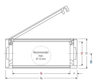
The maximum cable diameter strongly depends on the bending radius and the desired cable type. Please contact us.
