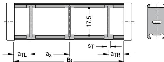
The dividers can slide along the chain cross section!
