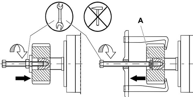
**Fig. 4 Pulling off and putting on output elements.**
