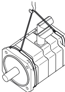
**Fig. 2 Lift and transport with suspension bands**
