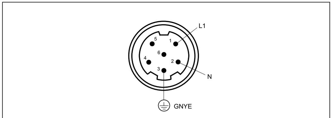
Figure 6-8 Connecting the separately-driven fan by means of the connector
