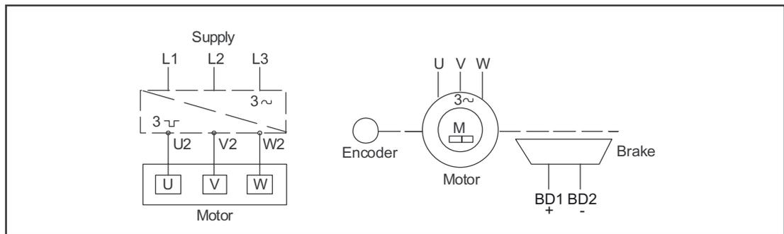
Figure 6-1 Circuit diagram
