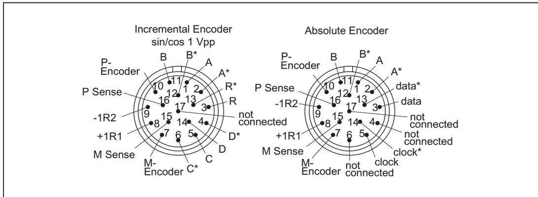
Figure 6-3 Signal connector (motor without DRIVE-CLiQ interface)
