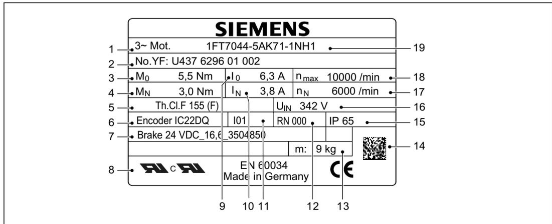
Figure 3-1 Schematic layout of rating plate
