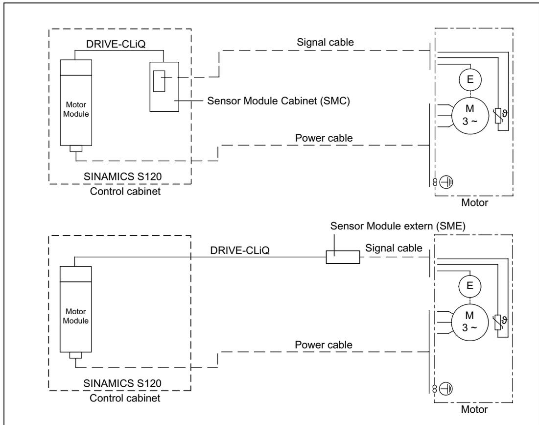
Figure 6-7 Encoder interface without DRIVE-CLiQ
