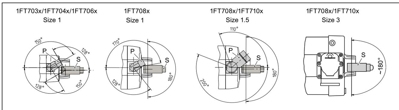
Figure 6-4 Ability to rotate the connectors (P = power connector, S = signal connector)
