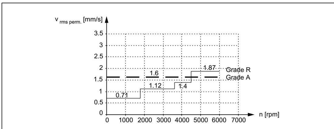
Figure 5-2 Vibration severity grades
